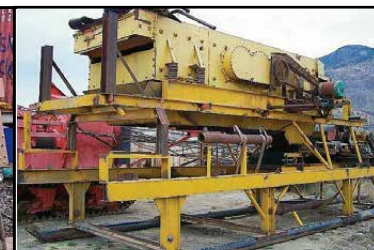
EL JAY 6 X 16 WASH SCREEN SKID MOUNT WITH SPRAY BARS
