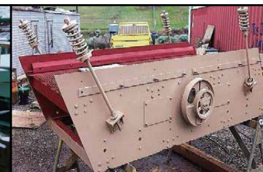
4X8 DILLON 2 DECK VIBRATING SCREEN
