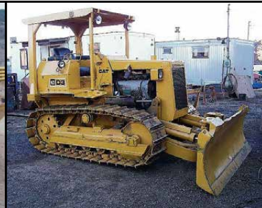
CAT D3 DOZER DEUTZ AIR COOLED DIESEL
