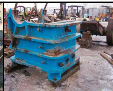
DISASSEMBLED 18" X 32" TELSMITH JAW CRUSHER
