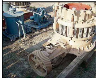
STANDARD & SHORT HEAD 24" SYMONS CONE CRUSHER
