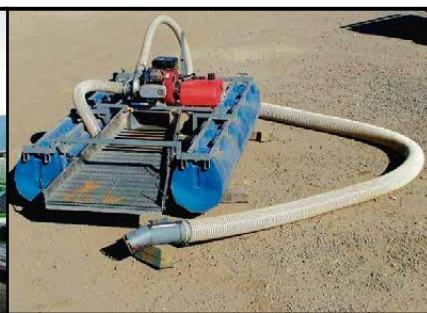
FLOATING DREDGE GAS DRIVE PUMP AND COMPRESSOR
